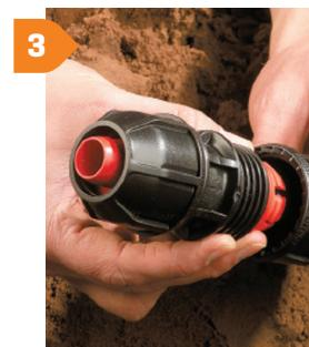
Push the insert into the body of the fitting, position the nut and grip ring and tighten by hand
